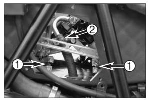
Dismounting the throttle body: remove both side covers on the air filter box, loosen the clamps • on the throttle body and dismount the fuel line •.
