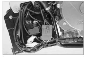
Connect the connector for the lambda probe, the side stand switch and the gear sensor to the wiring harness.
