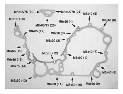
Screw in all HH case bolts (see illustration for bolt lengths) and tighten to 10 Nm.
