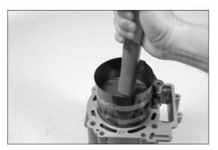
Use the hammer handle to carefully tap the piston into the cylinder, making sure the piston rings do not get caught.
