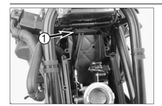
Mount the throttle cable duct ①.
