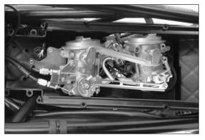
Pull the throttle body up, disconnect the wiring harness, remove both throttle cables and lift out the throttle body.
