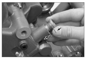
NOTE: measure the preload on the chain tensioner element before dismounting:
