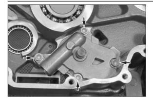
Apply Loctite 243 to the three remaining oil pump bolts (M6x40) and screw in. Tighten bolts to 10 Nm.
