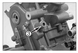
Mount the chain tensioner bolt 3 with a new sealing washer and tighten to 20 Nm.
