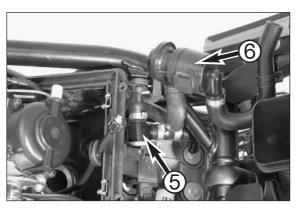
Mount the lower air filter box on the intake ports, connect the drain hose and push the fuel hose and the cable for the idle speed adjustment down through the opening in the lower air filter box.
