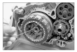
Insert a wire hook in the recess in the clutch disks and pull all of the clutch disks out of the clutch hub.
