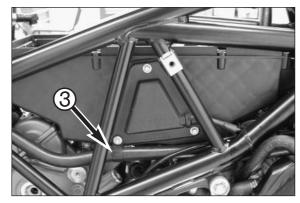
Screw on the right side cover of the lower air filter box together with the bracket 6 for the secondary air system hose.
