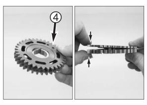
Mount the tensioning wheel so that the tension spring bolts engage in the right hole and then press the two gears together.
