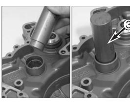
Place the bearing shells on the clutch cover with the assembling sleeve and press in the bearing shells to the stop using the press mandrel 600.29.046.028 ⑤.
