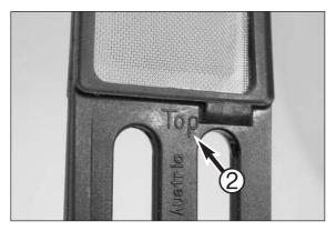
NOTE: the oil screen has a TOP marking 2 which must point up.
