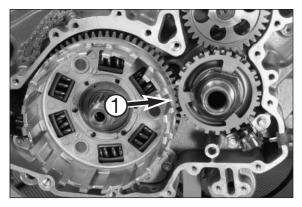
NOTE: you do not need to dismount the primary pinion if you are only replacing the outer clutch hub:
