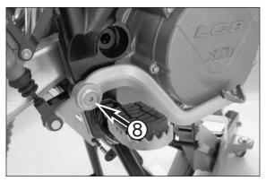
Position the foot brake pedal, apply Loctite 243 to the bolt 3 and tighten to 25 Nm.
