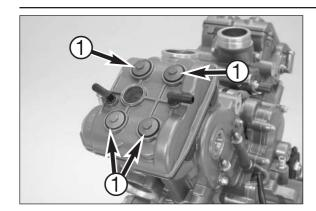
Clean the engine thoroughly on the outside prior to disassembling.
