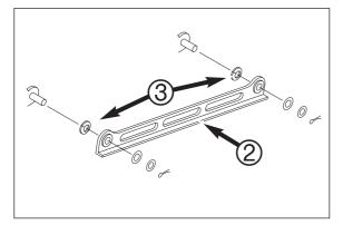
Mount the throttle linkage arm with shims as shown in the drawing and secure with the pins.
