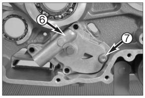
Mount the pressure pump case 3 and fix with the short bolt 4 (M6x25) (apply Loctite 243 to the bolt but do not tighten yet). Do not forget the centering pins on the pressure pump housing.
