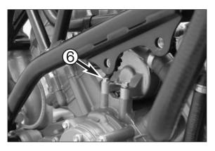
Screw on the ground cable terminal 6.
