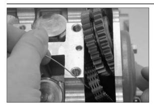
Push the double timing gear down into the chain tunnel draw the timing chain along the side on the inside.
