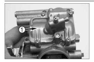
Remove the float chamber • and discard the gasket.
