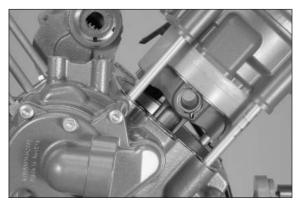
Pull the cylinder head and cylinder up until the piston-pin retainer can be lifted out of the groove on the clutch side with a suitable screwdriver.
