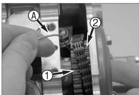
Use the wire hook ① to lift the side of the chain on the inside over the gear teeth ① onto the chain teeth ② of the double timing gear.
