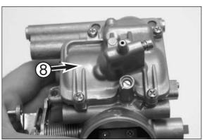
Mount the float chamber 3 with a new gasket. Tighten the screws.
