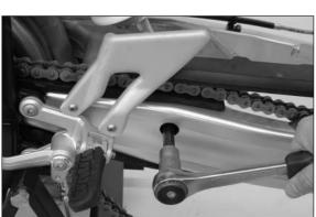
Remove the lower fork leg screw and press the swing arm down to release the fork leg out of the recess in the swing arm.
