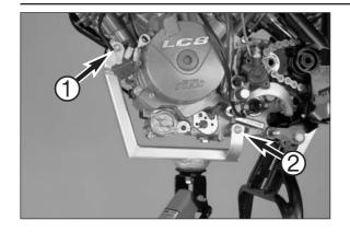
Use the trolley jack to position the attachment 600.29.055.100 on the engine, insert the bolt • through the front of the engine bracket and fasten with the nut. Screw one of the bolts • on the rear of the side stand fixture and slightly lift the engine.
