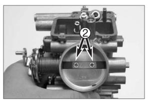
Mount the throttle valve ②, tighten and caulk the screws.
