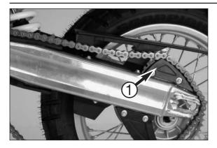
Unscrew the nut on the wheel spindle, pull out the rear wheel spindle, take the chain off of the rear sprocket and place over the side of the bracket ①. Remove the chain from the engine sprocket.
