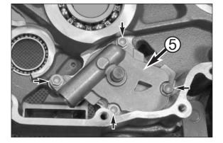
Loosen the bolts on the outer oil pump (pressure pump) and remove the oil pump housing.
