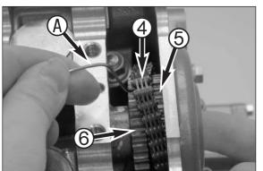
Use a wire hook which you can bend from a piece of welding wire to lift the side of the chain teeth towards the inside from the chain teeth over the gear teeth towards the double timing gear. Hold the double timing gear towards the outside by inserting your finger through the hole in the bearing bolt.
