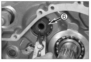
Bring the engine into a vertical position (mounting position) and remove the lock ring 6 and washer from the countershaft.
