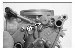
Unscrew the ACV cover 6 and remove the spring 6 together with the diaphragm 7.
