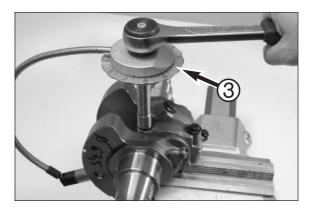
Tighten the conrod bearing bolts with the special wrench socket 600.29.075.000 to 25 Nm (1st stage). The tighten to 30 Nm (2nd stage) and finally by another 60° (3rd stage).
