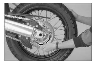
To check the jerk damper: hold the rear wheel while you try to move the rear sprocket back and forth in the running direction.
