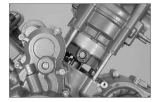
Pull the cylinder head and cylinder up until the piston-pin retainer can be lifted out of the groove on the generator side with a suitable screwdriver.
