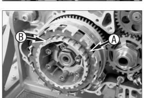
Slide the 25 x 48 x 6.5 mm disk and inner clutch hub together with the clutch pressure booster onto the main shaft teeth.
