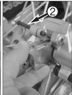
Slide the left brake pad into the brake caliper and fix with the bolt.
