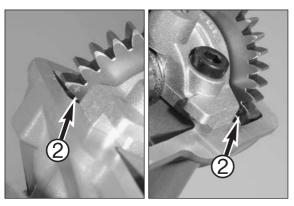
Turn the crankshaft in a counterclockwise direction until the rear cylinder is in the TDC position. The marks ② (crosses) must coincide with the flat outer surface of the cylinder head at the camshaft gears.
