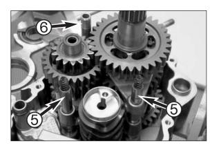
Mount the gearshift rails 6, paying attention to the lower gearshift rail springs. Insert the upper gearshift rail springs in the gearshift rails with the tapered ends up.
