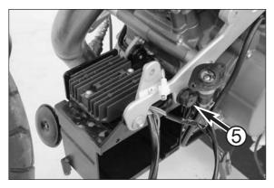
Mount the battery case with the controller and horn, using the black screw 5 in the position shown.
