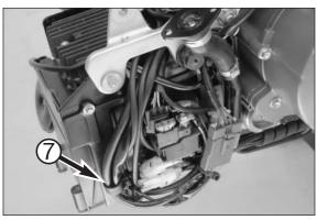
Align the wiring harnesses in a loop as shown in the photo and fasten with clamp of and cable clips.
