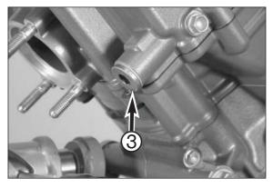
Mount the chain tensioner bolt 3 and tighten to 20 Nm.
