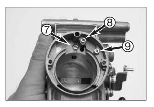
Mount the main air jet **7**, ACV jet **3** and idle-air jet **9** with a suitable screwdriver.
