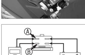
Connect the auxiliary starter relay (see drawing) to a 12 V battery, making sure you hear the relay switch (nonrecurring "click").
