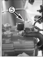
Connect the connectors for the oil pressure switch ③, the temperature sensor ④ and the front ⑤ and rear ignition coil. Secure the wiring harnesses with cable clips.
