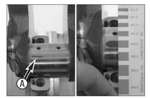
Clamp each conrod in a vise, insert new bearing shells, position the crankshaft with a plastigauge measuring strip (600.29.012.000) on top and mount the conrod caps with the old bolts, as described below.
