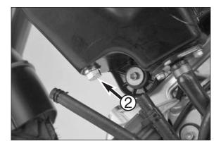
Unscrew the oil drain plug ② on the oil tank and allow the oil to drain into a receptacle.
