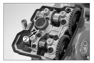
Dismount the gaskets of the bolts, the valve covers and the spark plug shafts ②.
