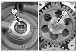
Turn the water pump shaft 3 until the recess fits over the driver 4 of the balancer shaft when the clutch cover is mounted.
