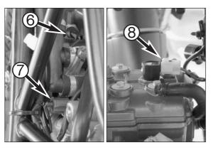
Detach the connector from the oil pressure switch ⑤, the temperature sensor ⑦ and from the front ⑥ and rear ignition coil. Remove any cable clips necessary.
