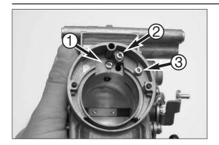
Unscrew the main air jet ①, the ACV jet ② and the idle-air jet ③ with a suitable screwdriver.
