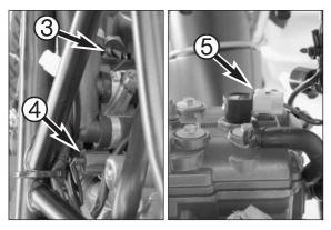
Plug the connector on the oil pressure switch (3), the temperature sensor (4) and the front and rear ignition coil (5). Use cable clips to fasten the wiring harnesses.
