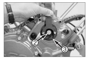
Hold the water pump wheel with special tool 600.29.082.000, remove the bolt and pull the water pump wheel off of the shaft.
