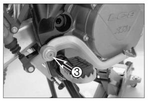
Remove the bolt 3 and tilt the foot brake pedal to the side.
