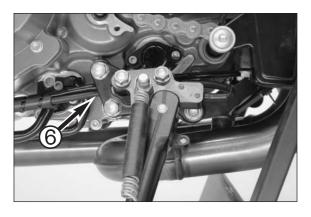
Position the side stand and tighten both screws and the nut to 45 Nm (+ Loctite 243).
