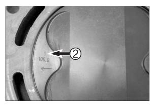
The piston size ② is impressed in the top of the piston; 1 is size I, 2 is size II.
