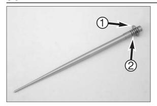
Mount the lock ring 1 in the respective position on the jet needle
