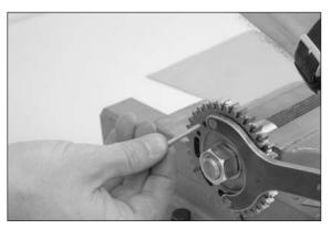
Apply the pretensioning tool hook wrench 600.29.051.000 to the tensioning wheel and turn against the spring until the pin can be inserted in the hole.
