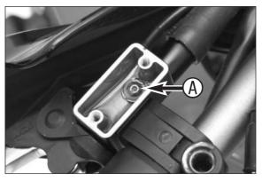
Refill oil, until oil is discharged from the bore **3** of the master cylinder in a bubble-free state. Make sure that the oil does not overflow.
