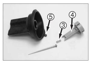
Insert the spring 3 in the jet needle holder 4 and position in the throttle slide together with the jet needle. Clip the jet needle holder into place.
