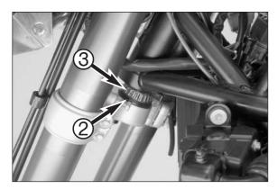
Clean the gasket element ② and grease the lower steering head bearing ③.
