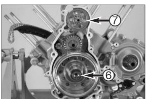
Mount the rotor bolt with disk, apply Loctite 243 to the bolt and tighten to 180 Nm (M16) or 150 Nm (M16x1.5).
