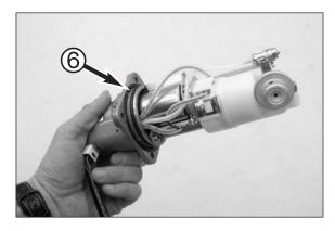
Remount in the reverse order, always replacing the O-rings 6 for the fuel pump and fuel connector.
