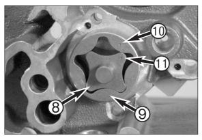
Insert the needle roller in the oil pump shaft and slide on the inner rotor 3 of the suction pump. Mount the outer rotor 9 such that the mark 10 is visible on the outside.
