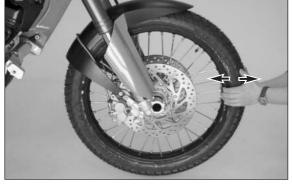
If you feel any clearance, loosen the 5 clamp bolts on the top triple clamp and turn in the blind nut • until no clearance is left.
