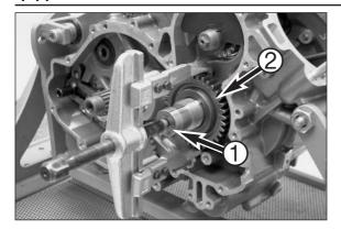
Insert the pressure tool 600.29.031.000 **1** in the crankshaft bore, turn the balance weight up and pull the primary pinion **2** off the crankshaft with the puller 600.29.033.000.
