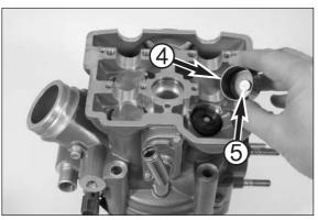
Mount the bucket tappets 4 and the valve shims 5 in their original positions in the cylinder head.
