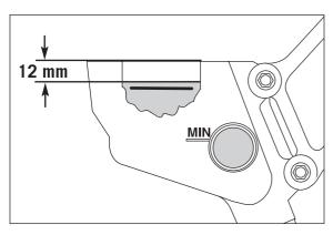
Add DOT 5.1 brake fluid (Motorex Brake Fluid DOT 5.1) up to 12 mm under the top edge of the reservoir. Remount the rubber boot, cover and screws. Wash off any overflowing or spilled brake fluid with water.
