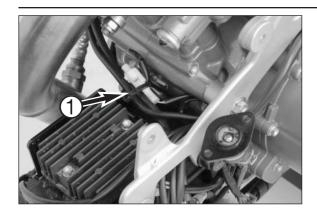
Fasten the wiring harnesses and connector on the pulse generator
