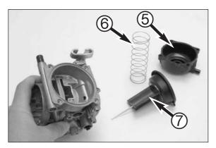
Remove the throttle slide spring 3 and pull the throttle slide 0 out of the carburetor together with the diaphragm.
