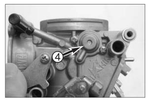
Place the spring on the diaphragm and mount the ACV cover 4.
