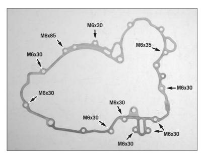
Mount the dowel pins on the engine case and put a new clutch cover gasket in place.
