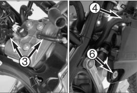
Pull off the oil lines from the oil tank to the valve covers 3 and the return line 4 (special pliers 600.29.57.100), unscrew the oil lines from the oil terminal 5 and pull out. Remove the O-rings.
