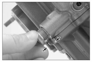
The measured value should be between 6 mm and 11 mm. If the value is lower, the tensioning rail could be worn or the timing chain excessively elongated. If it is higher, the engine was turned to TDC against the running direction.
