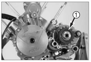
Mount the engine sprocket with the lock washer and tighten the nut
