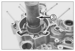
Press in the bearings from the outside to the inside through the assembling sleeve up to the stop using the press mandrel 600.29.044.050 3.
