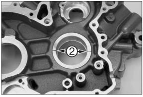
Position the bearing shells on the output end of the case such that the end gap on the bearing shells points to the marks 2 made when disassembling.
