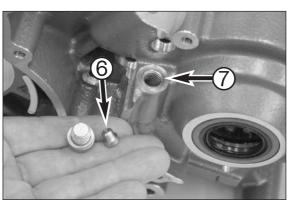
Remove all shaft seal rings and the dowel pins from the case halves.
