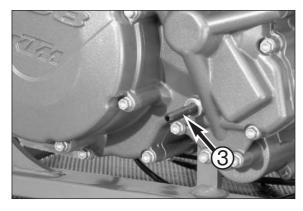
Remove the case bolt and screw in the special tool 0113 080802
