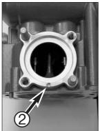
Invert the cylinder head, mount a new cylinder head gasket and put the cylinder into position.
