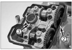
Mount the valve cover gaskets 2 and spark plug shaft gaskets 3.
