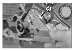
Remove the inner oil pump 6 (suction pump).
