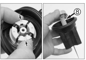
Press the jet needle holder 3 together in the direction of the arrows, carefully unclip from the jet needle and remove.
