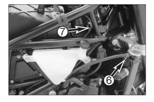
Mount the radiator compensating tank, connect the short hose 6 to the radiator, run the longer hose 7 in front of the intake snorkel over the air filter box to the left side of the motorcycle and continue along the frame to behind the battery case.
