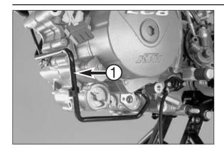
Mount the front oil line ● inserting new O-rings. Tighten the bolts.
