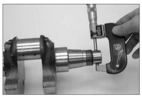
Measure the diameter of the bearing pin at 3 points that are 120° apart using a micrometer gauge.
